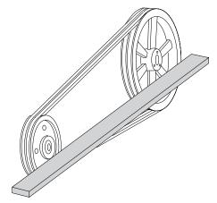
Aligning sheaves with a straight edge
